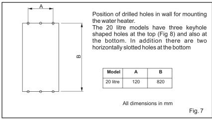
panel and if this is a suitable height then with the water heater still in position, mark out the screw hole positions for the two bottom slotted mounting holes.
